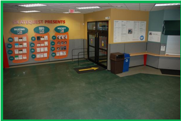
Figure 20. EFFECTIVE – This camera position shows the approach to the door. The height and angle of the camera are optimal for event detection. Since the door is glass, the fact that the camera is not facing it will minimize the effects of reflections on the glass.
