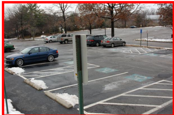
Figure 39. INEFFECTIVE – A sign in the foreground obstructs part of the camera view.
