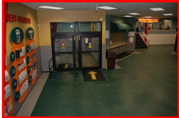
Figure 21. INEFFECTIVE – The camera is directly facing the glass door, which can reflect light.
