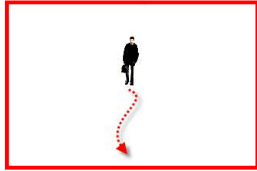
Figure 6. LESS EFFECTIVE – A target near the camera traveling directly toward the camera spends less time in the camera view and changes size rapidly.
