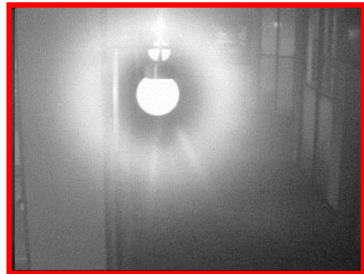
Figure 18. INEFFECTIVE – Light completely obstructing the camera view.
