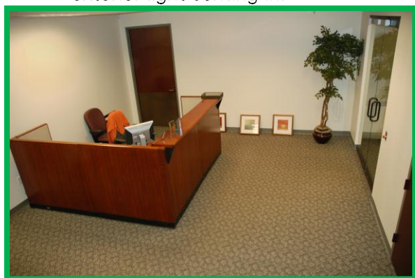
Figure 28. EFFECTIVE – This camera is mounted at the entrance of an office suite to monitor people who enter the suite after hours. The camera is mounted at an appropriate angle, height, and distance from people coming into the room. While the camera view includes a glass entry door, the fact that the camera is not directly facing it minimizes the risk of unwanted event notifications due to reflections or lighting.
