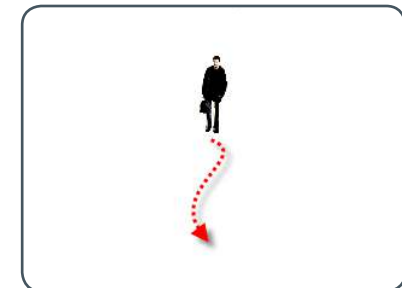
B LESS EFFECTIVE - A target traveling directly toward the camera
