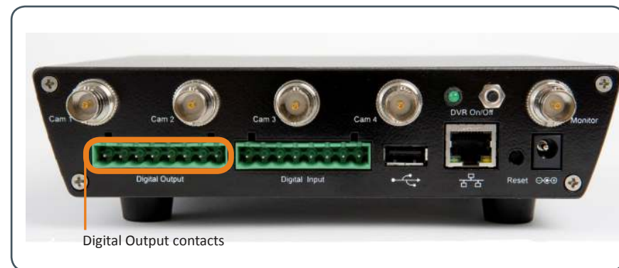
Figure 31 Digital Output contacts on CheckVideo Gateway
