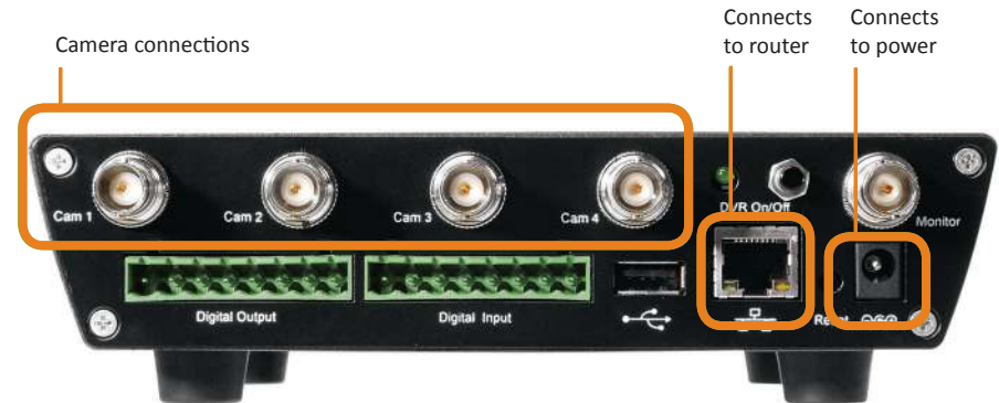
Figure 1 Back panel of the CheckVideo Gateway
