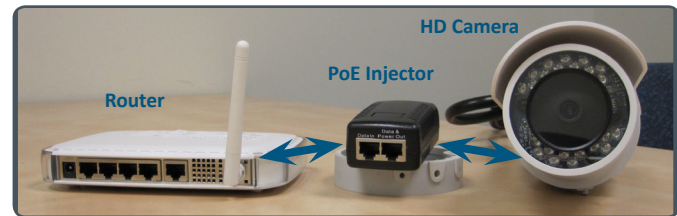
Fig. 1a- Connection path using a PoE injector as the mid span
