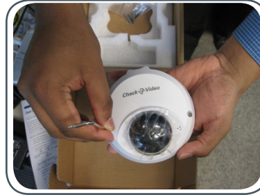
Fig. 5 - Remove the cover using the supplied hex wrench
