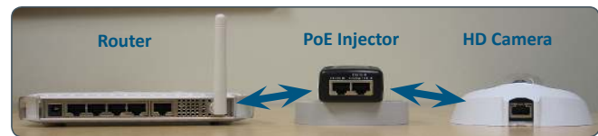
Fig. 1 - Connection path using a PoE injector as the mid span
