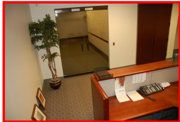
Figure 29. INEFFECTIVE – The camera is directly facing the glass door at the entrance (see page 19).
