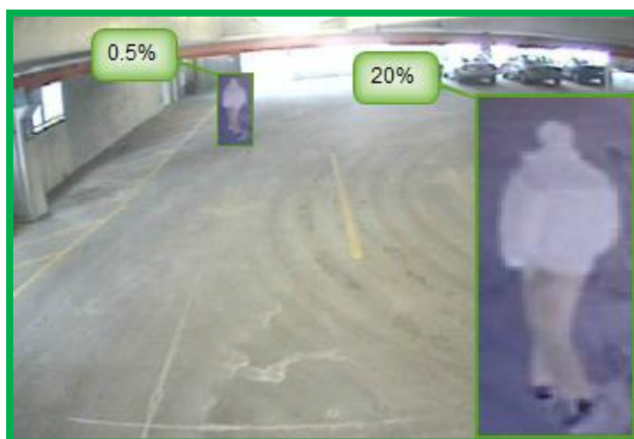
Figure 4. EFFECTIVE – Two targets within the detection range (taking up 0.5% and 20% of the view).
