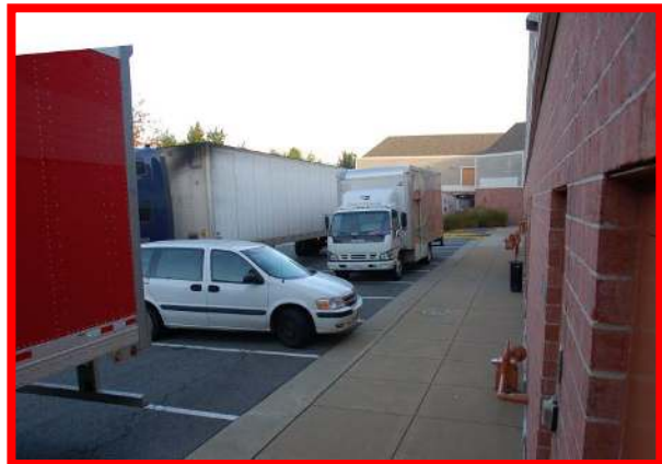
Figure 34. INEFFECTIVE – Several parked vehicles obstruct the camera's view of the entire camera view.
