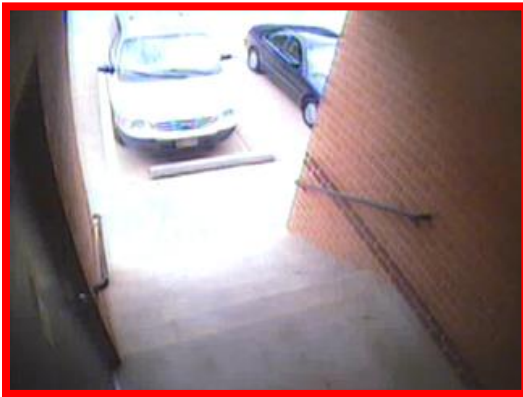
Figure 12. INEFFECTIVE – This camera view includes too much contrast between the darkened hallway and the glare of light from the outside.
