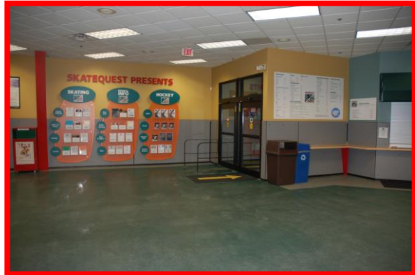
Figure 22. INEFFECTIVE – The camera is mounted too low, providing a 0° angle (see page 6).
