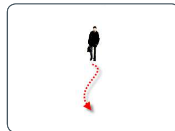
LESS EFFECTIVE - A target traveling directly toward the camera
