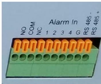
The ExpressHD Gateway has 4 Input pins and 1 Output pin along with 1 ground pin.
