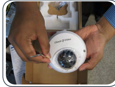
Fig. 4 - Remove the cover using the supplied hex wrench
