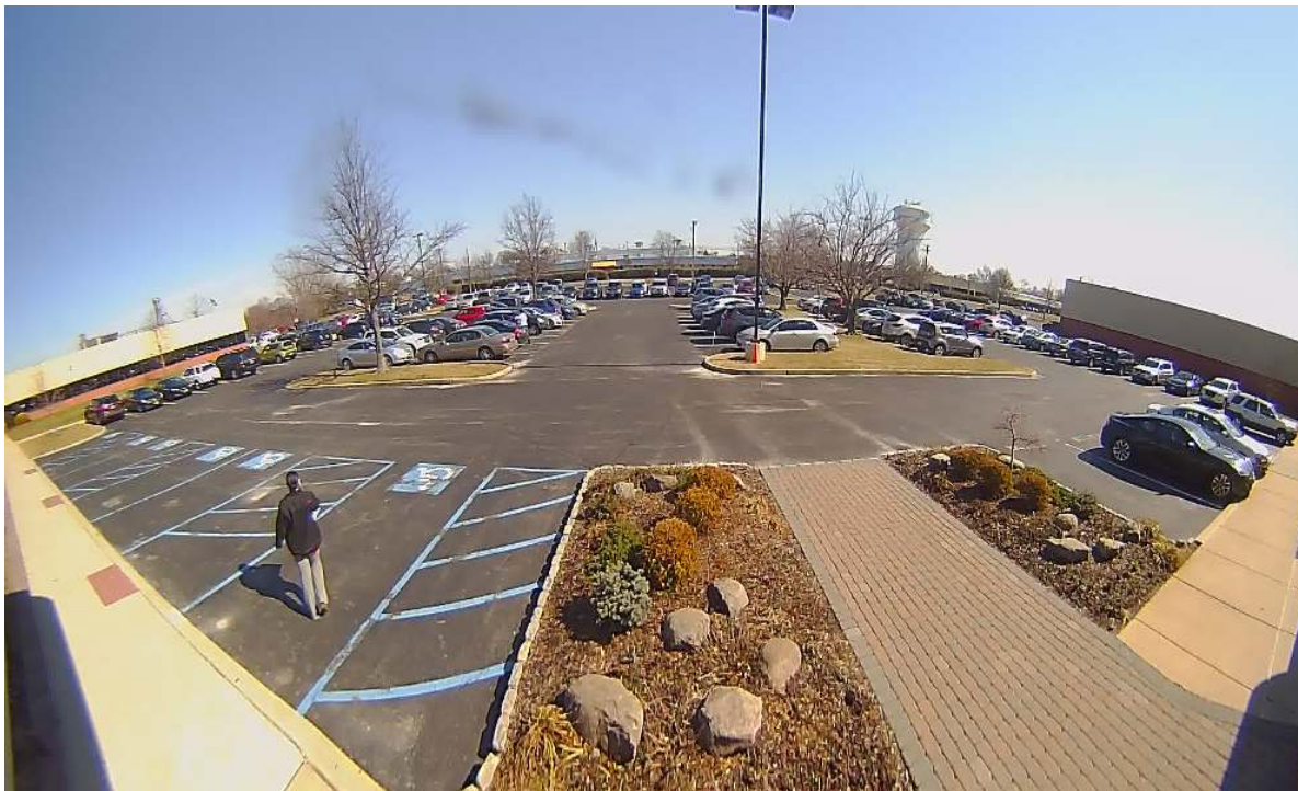
Panoramic image from CV181 The camera is mounted 15ft high using a 20 degree mount
