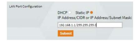
**IMPORTANT:** Note that the above is simply an example provided cameras use IP addresses in the range 192.168.1.x. If cameras are already assigned IP addresses, they may not be in the range 192.168.1.x. They may use a different base address such as 10.1.2.x in which case the entry for the
