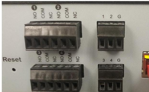
The CV4IP-16-12T Gateway has 4 Input pins and 4 Output pins, along with 2 ground pins, one per 2 Input pins.
