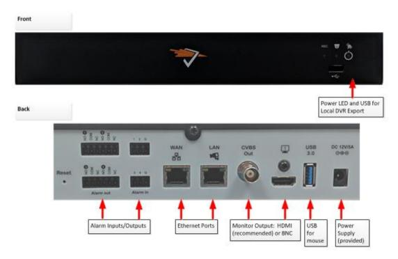
To install the Gateway, make the following connections to the CV4IP16:
