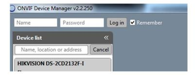
Select the camera from the list of visible cameras on the left side of the screen. Click on the Video Streaming link.
