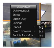
• Once the layout is selected, assign a camera to each window. Right-Click on the desired location to highlight the window orange. Right-Click again for the Menu and choose Select Camera. A list of cameras associated to the CV4IP will display for selection. Once selected, the camera's Live view will appear.
