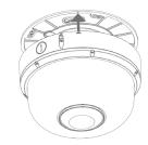
Twist the camera counterclockwise until it is secured firmly in place. Then fix the camera on the ceiling with the screw.
