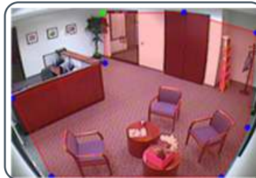
A zone, defined by eight end points (first point is green; other points are blue)
