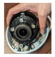
If attaching to brick or drywall, insert the 6. plastic expansion screw sleeve in the wall/ceiling. In all instances, place the Oring on the provided self-tapping screw (or the provided M4x0.7 machine screws, if using a mount kit), insert the screw in the camera body's mounting holes and screw the camera in place. Note that extra O-rings will be provided in case one is lost during install.
