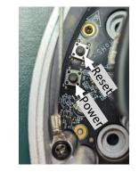
The cable closest to the security cable is for a camera Reset. This is equivalent to a power cycle. To complete the reset, press and release the button.
