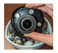
8. Next adjust the angle/tilt. The optimal angle for analytic detection is between 15 and 45 degrees. Loosen the side screws in a counter-clockwise manner. Tilt the ball and tighten the screws once the proper angle is achieved.
